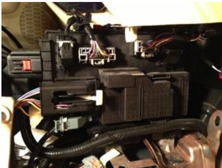
*Figure 1: Chassis Computer (SJB) from a 2010 Ford Escape*
