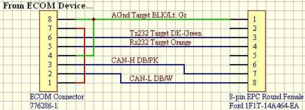
Figure 10. Ecom cable schematic
