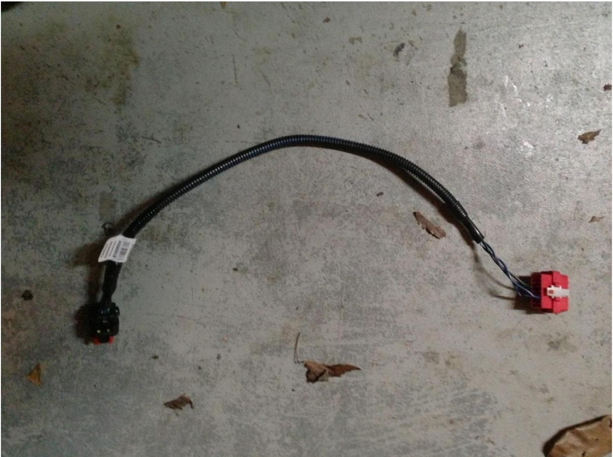
Figure 11: Handmade ECOM-OBD-II connector
