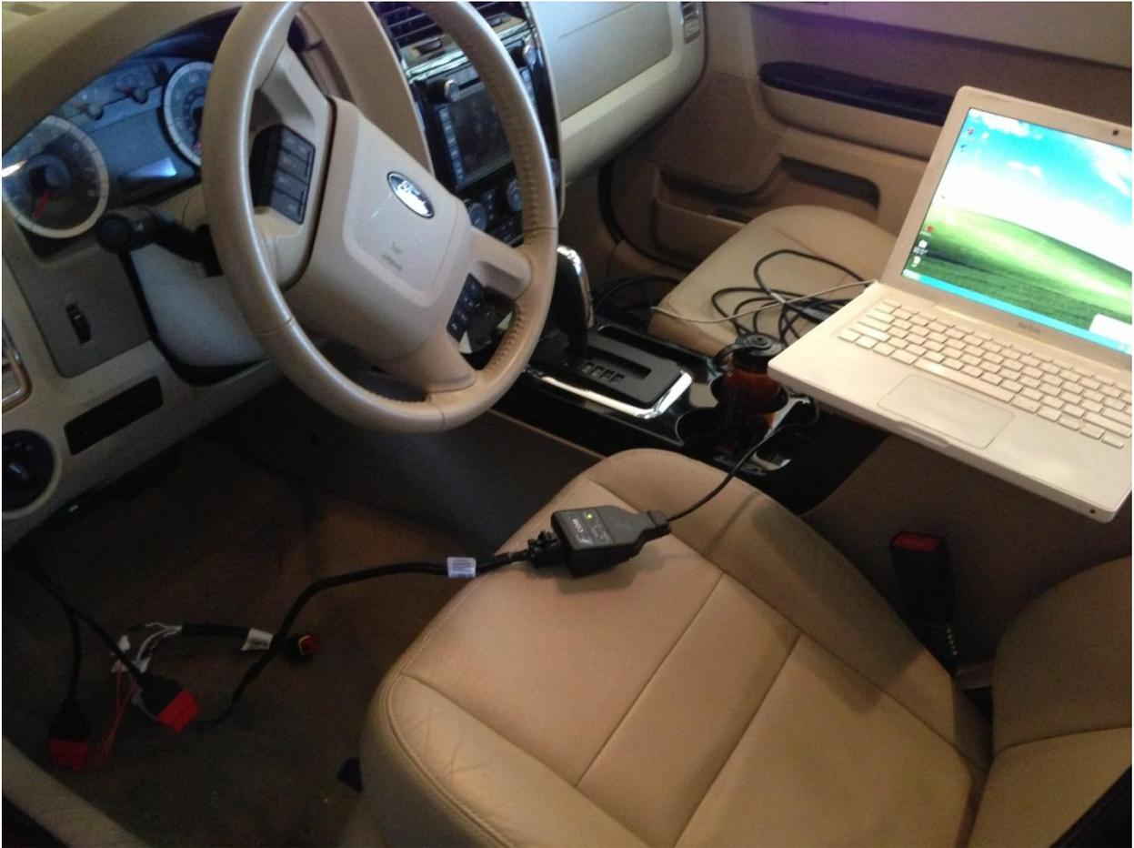
*Figure 12: A laptop communicating with the CAN bus*
